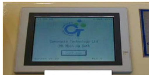
The bath is designed to be fully automatic although some of the operations can be done manually. Manual control of the water fill valve, the water drain valve and each motor stirring bank are all possible. Installation of the CT4 is quick and easy. A competent fitter can carry out electrical and mechanical connection.
